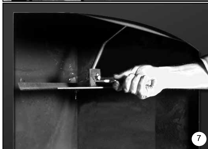
Figure 18b: Installation de la trousse catalytique
